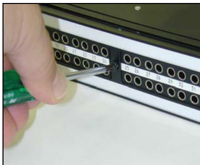
\partial Remove Front Panel
