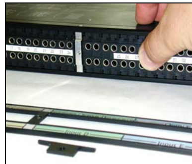
\bullet Pull out channel ID strip
