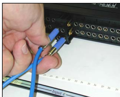
Alternative way to pull out module
